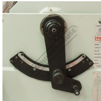
Rapid Blade Adjustment for Material Thickness
