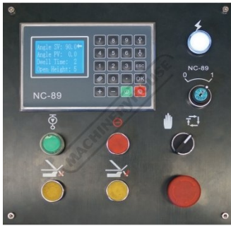
NC 89 Control Panel
