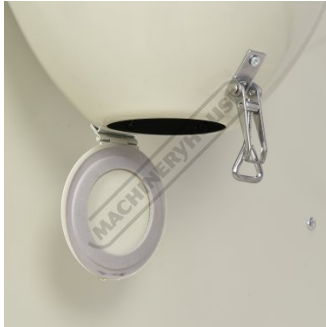
Dust Collector Emptying Hatch
