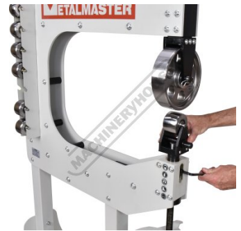
Lower Wheel Release Bolt Action
