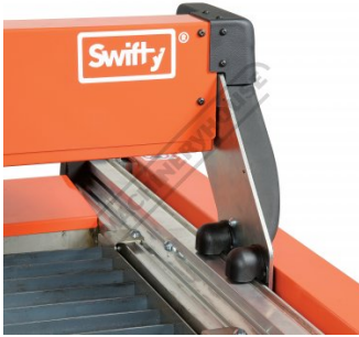
Gantry Roller Support Right View
