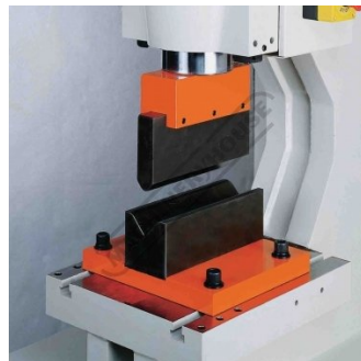
Optional Single Vee Pressbrake Attachment
