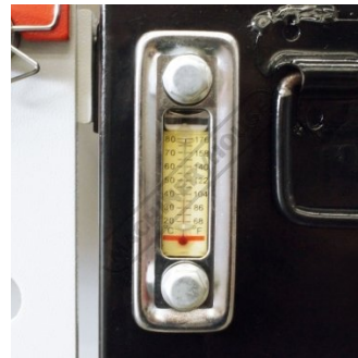
Hydraulic Oil Level Gauge
