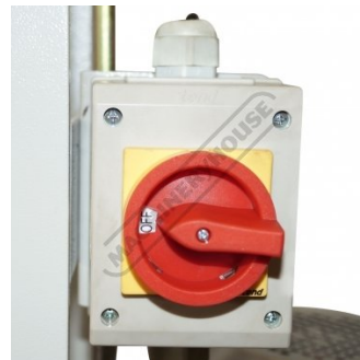
Main Power Isolation Switch
