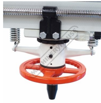
Quick Action Hand-Wheel for Rapid Approach
