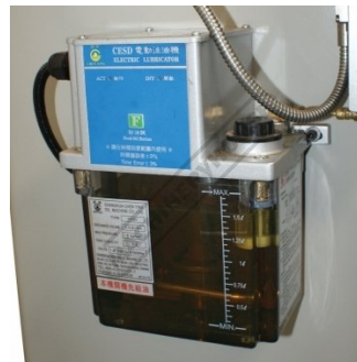
Automatic oil lubrication pump and reservoir
