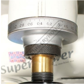
Metric dial graduations for X Y & Z Axis
