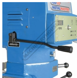
Spindle Brake Lever
