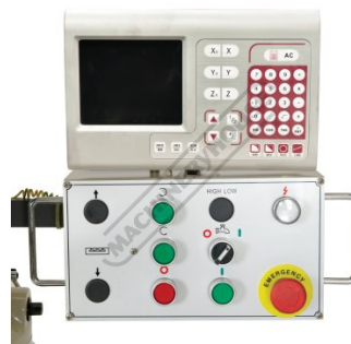
Control Panel & 3 Axis Digital Readout
