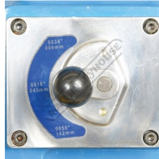
Feed Speed Selector Lever
