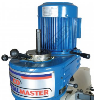
Spindle Break Lever High or Low Speed Selector and Belt Tension Handle
