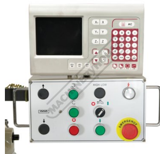
Control Panel & 3 Axis DRO with X & Y Axis Scales
