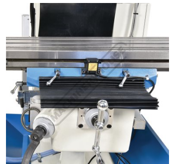
Coolant Hose Table Feed Limit Switches
