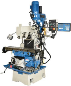
Removed Dividing Head Horizontal Head Setup
