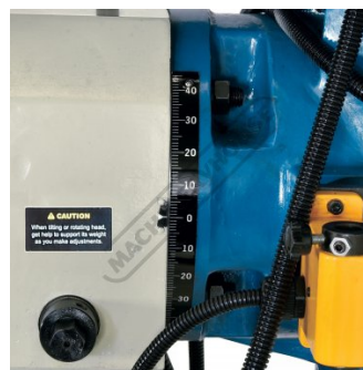
Tilting Mill Head Left & Right to 90 Degrees
