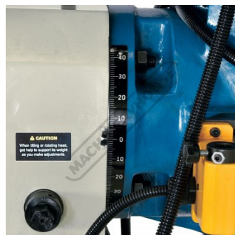
Tilting Mill Head Left & Right to 90 Degrees
