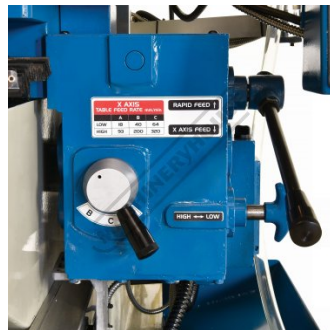
Gear Drive Table Feed
