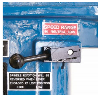
High Low Spindle Speed Gear Lever
