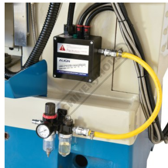
Air Powered Draw Bar System
