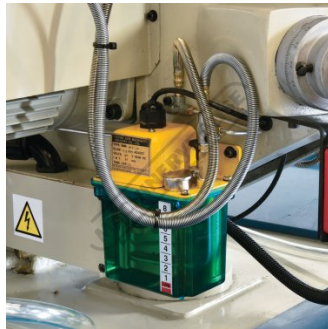
Automatic Slideway Lubrication System
