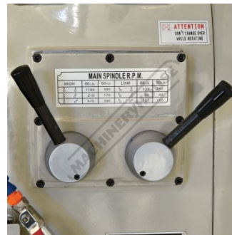
Horizontal Speed Selection Levers
