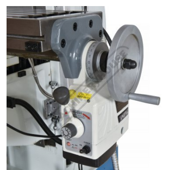
X Axis Power Feed With Rapid
