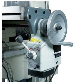
X Axis Power Feed with Rapid
