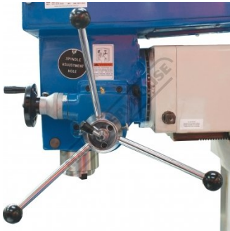
Quill Feed Handle and Fine Feed Dial
