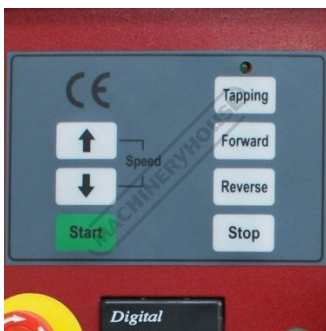
Spindle Control Panel
