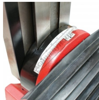
Milling head Tilts 45 Degrees both directions
