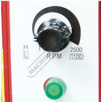
Electronic variable speed system
