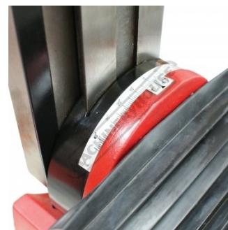
Milling head Tilts 45 Degrees both directions
