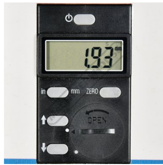
Digital Readout on Quill Depth
