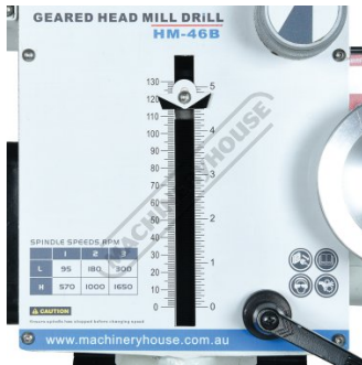
Quill Depth Stop Scale-Spindle Lock
