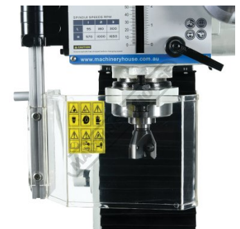
Interlocked Spindle Safety Guard
