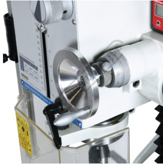
Fine Quill Feed Handwheel
