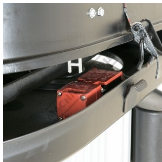
Safety Micro Switch on Belt Guard
