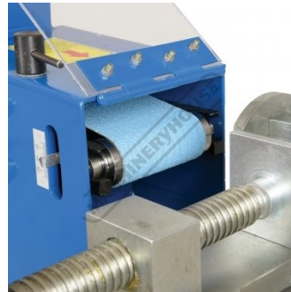
Includes 1 Roller Suitable for 32mm NB Pipe or 42mm Tube
