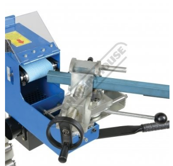
Square Vice Jaws Holding Material at 45 Degrees 2
