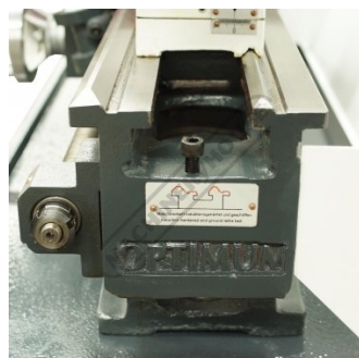
Induction Hardened and Ground Bed
