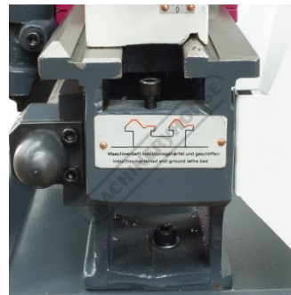
Induction Hardened and Ground Bed
