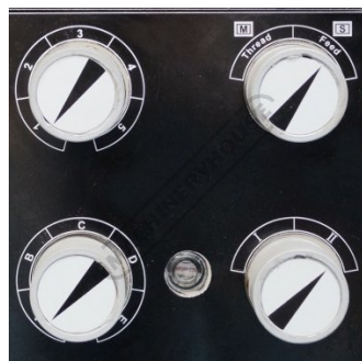
Feed and Thread Gearbox
