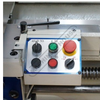
Saddle Switch Board
