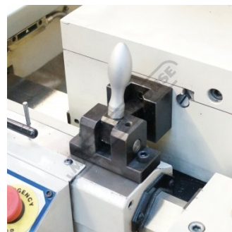
Tailstock Moving Device Locked Position
