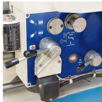
Saddle Feed Controls
