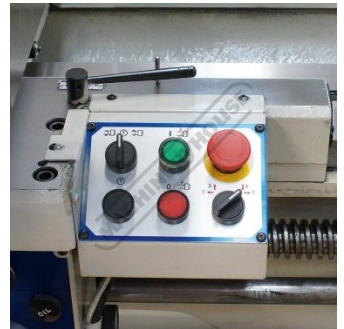
Saddle Switch Board
