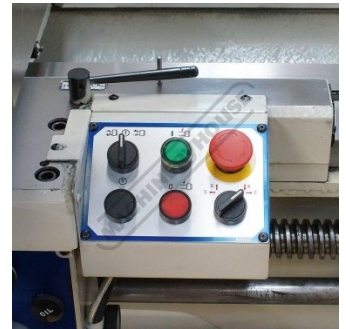
Saddle Switch Board
