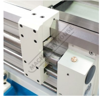
Moveable Leadscrew and Feed Shaft Support
