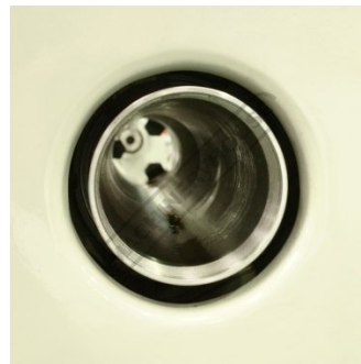
80mm Spindle Bore
