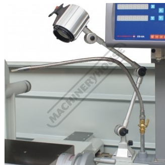
Coolant Nozzle and LED Work Light
