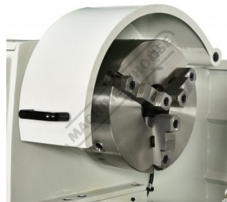
Safety Chuck Guard
