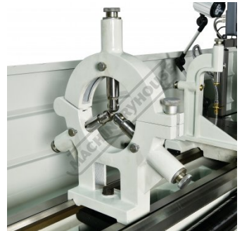
Fixed Steady with Roller Bearings
