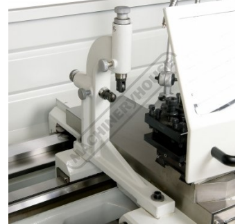
Travelling Steady with Roller Guides
