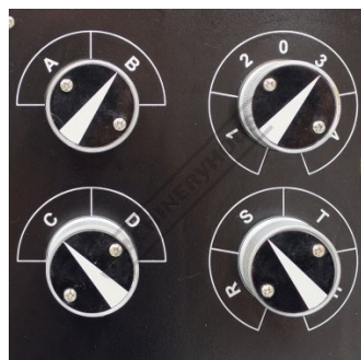
Gearbox Feed Controls
