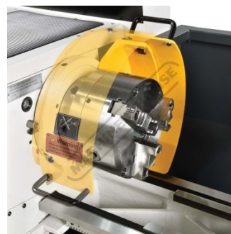
Chuck Guard with Safety Micro Switch
