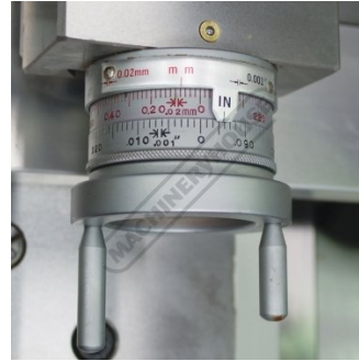
Compound Slide Dial - Dual Calibrated
