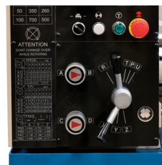
Enclosed Quick Change Gearbox
