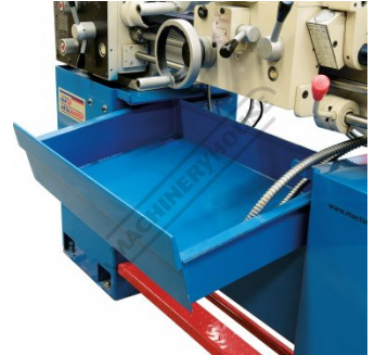
Sliding Drip Tray for Swarf Removal
