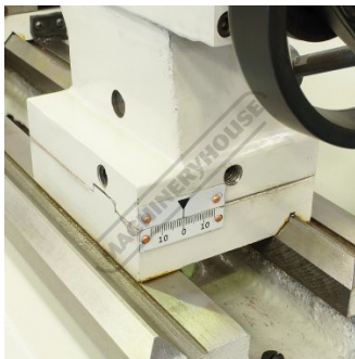
Tailstock Horizontal Adjustment
