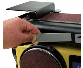
Releasing Tension To Change Belt
