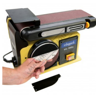
Removing Sanding Disc & Lower Guard
