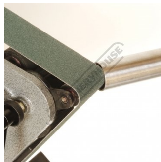
Internal Pipe Chamfering
