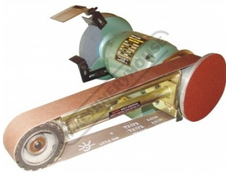
Shown Fitted to a Optional Bench Grinder
