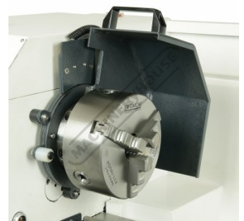
Safety Chuck Guard Open Position
