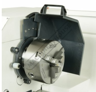
Safety Chuck Guard Open Position
