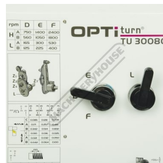
Spindle Speed Levers and Speed Chart
