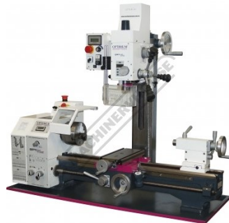
Toolpost Removed for Milling Application
