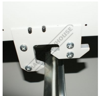
Drawer in Unlock Position
