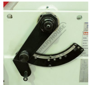
Rapid Blade Adjustment for Material Thickness
