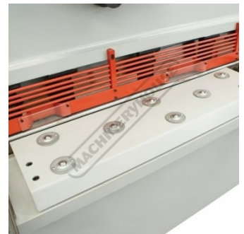
Material Transfer Balls On The Table
