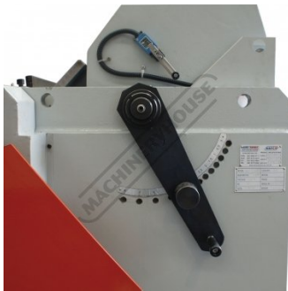
Rapid Blade Adjustment For Material Thickness
